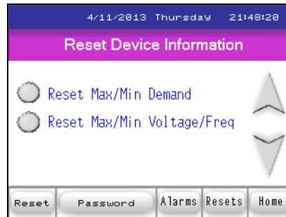
FIGURE 10-36: Three Phase/Single Phase Reset Device Information screen
