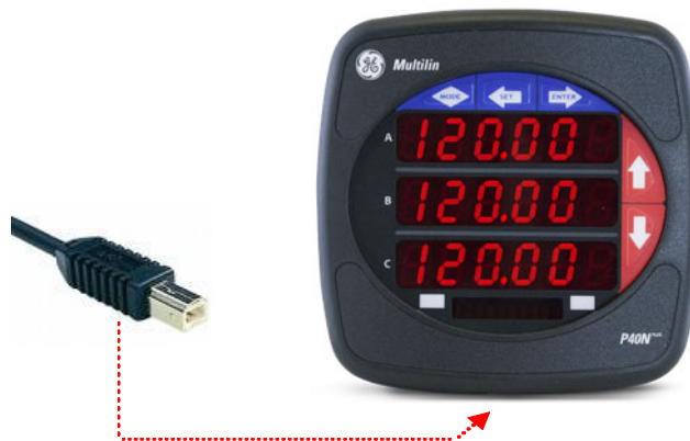
Figure 5-1: USB-B Male Connector and P40N PLUS USB Port
