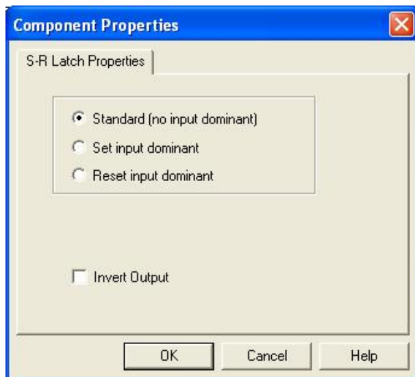
Figure 5: SR latch properties
