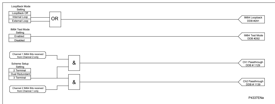
Figure 33: InterMiCOM 64 general alarm signals (conceptual logic)
