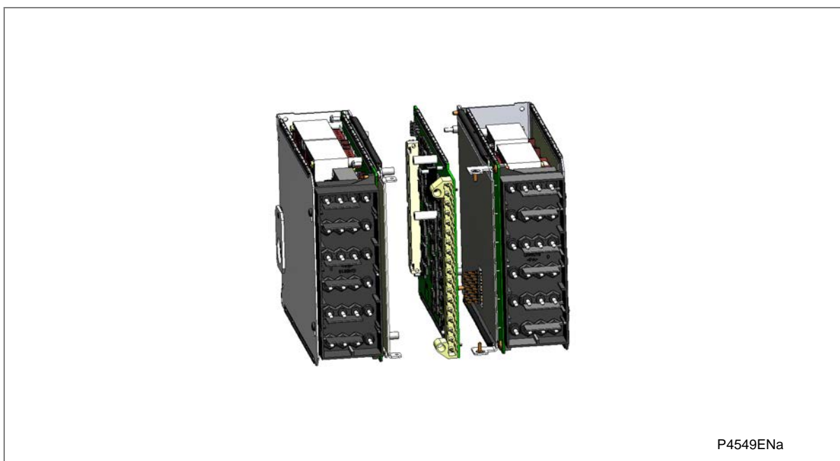
Figure 16: Input module with two transformer boards
