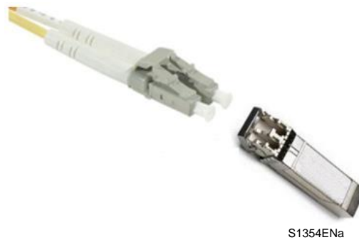
Figure 37: Ethernet Fiber Optic – LC-type Module
