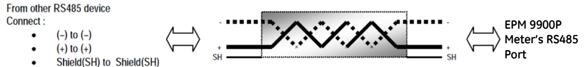
Figure 5-2: 2-wire RS485 Connection
