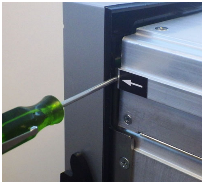
Figure 2-11: Unlatch Module (location is marked by arrow)
